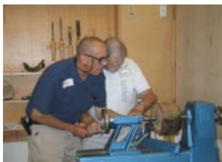
Winding the tailstock is a two hand operation
